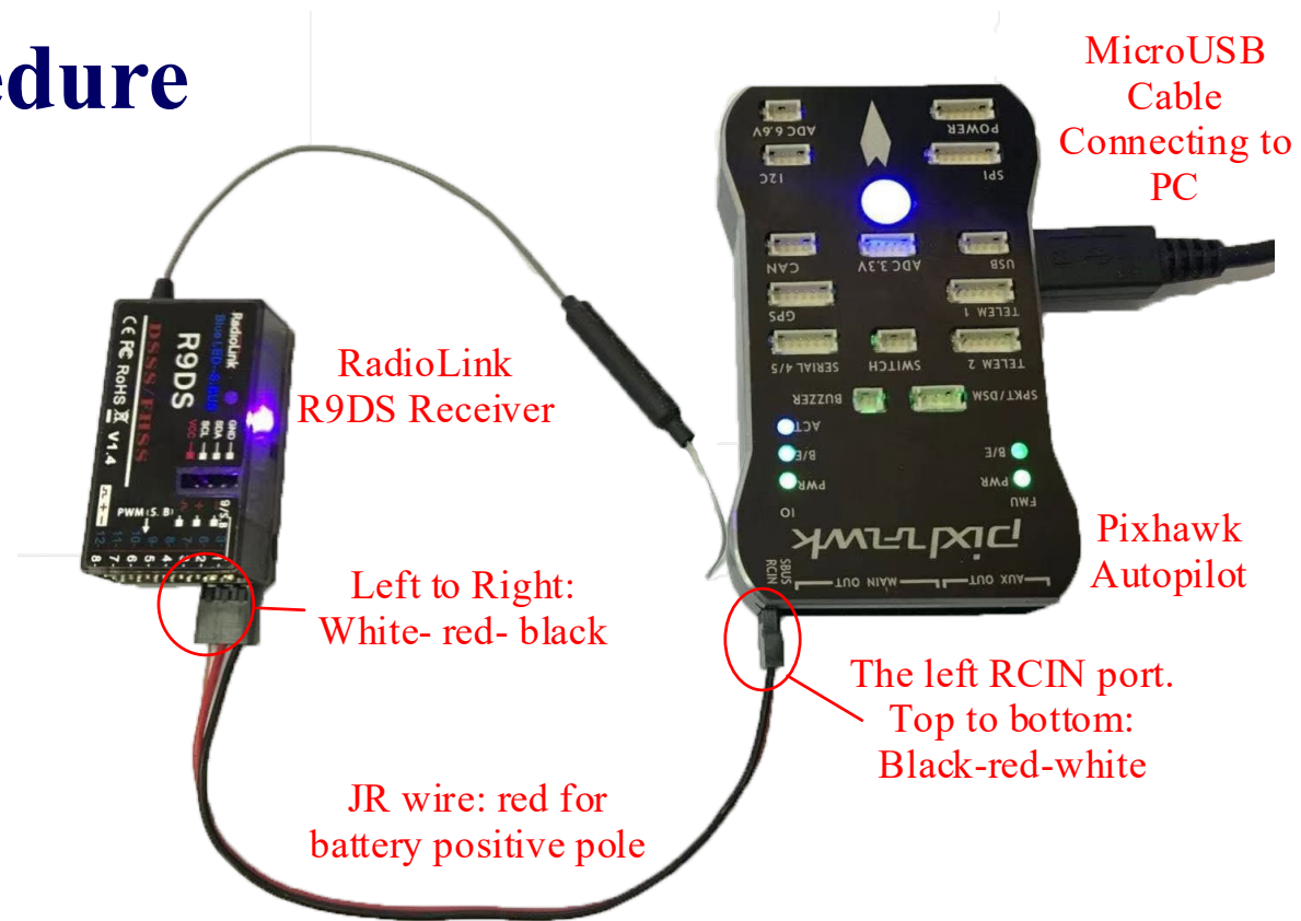
Figure. Connection between Pixhawk hardware and RC receiver
