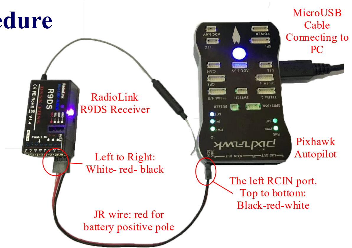
Figure. Connection between Pixhawk hardware and RC receiver
