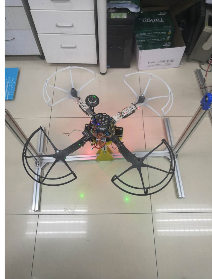
Figure. A quadcopter on a test stand
