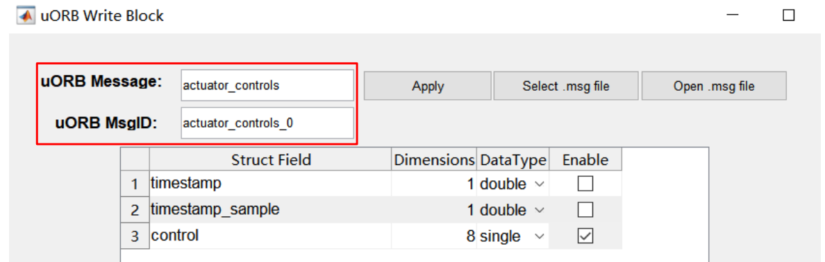
(b) uORB Write Advanced_dai module. uORB MsgID can be set different from the name of the “.msg” file.
