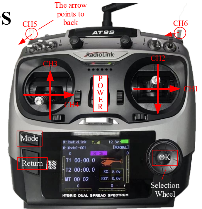
Note: the arrows point to the increasing direction of PWM
